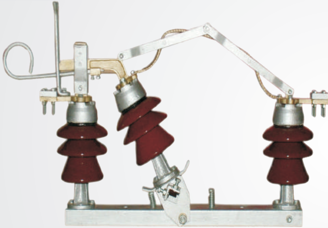
11/22/33 KV Outdoor triple pole Three insulator per pole tilting type, Gang Operated Air Break Switch Suitable for horizontal / vertical mounting with complete operating mechanism. Test as per IS-9920 / 1985
